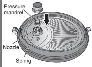
Before installing the nozzle cap, make sure there is no oil or blocking on the nozzle cap, nozzle and pressure mandrel.
