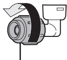
Hose clamping nut (Turn to remove) 鎖緊水管用螺帽 (旋轉後取出)
