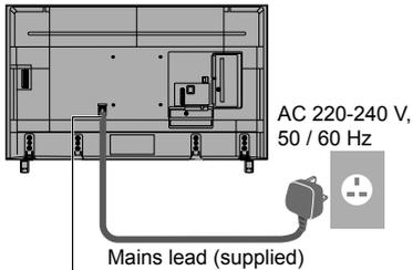
Insert the mains plug firmly into place.
